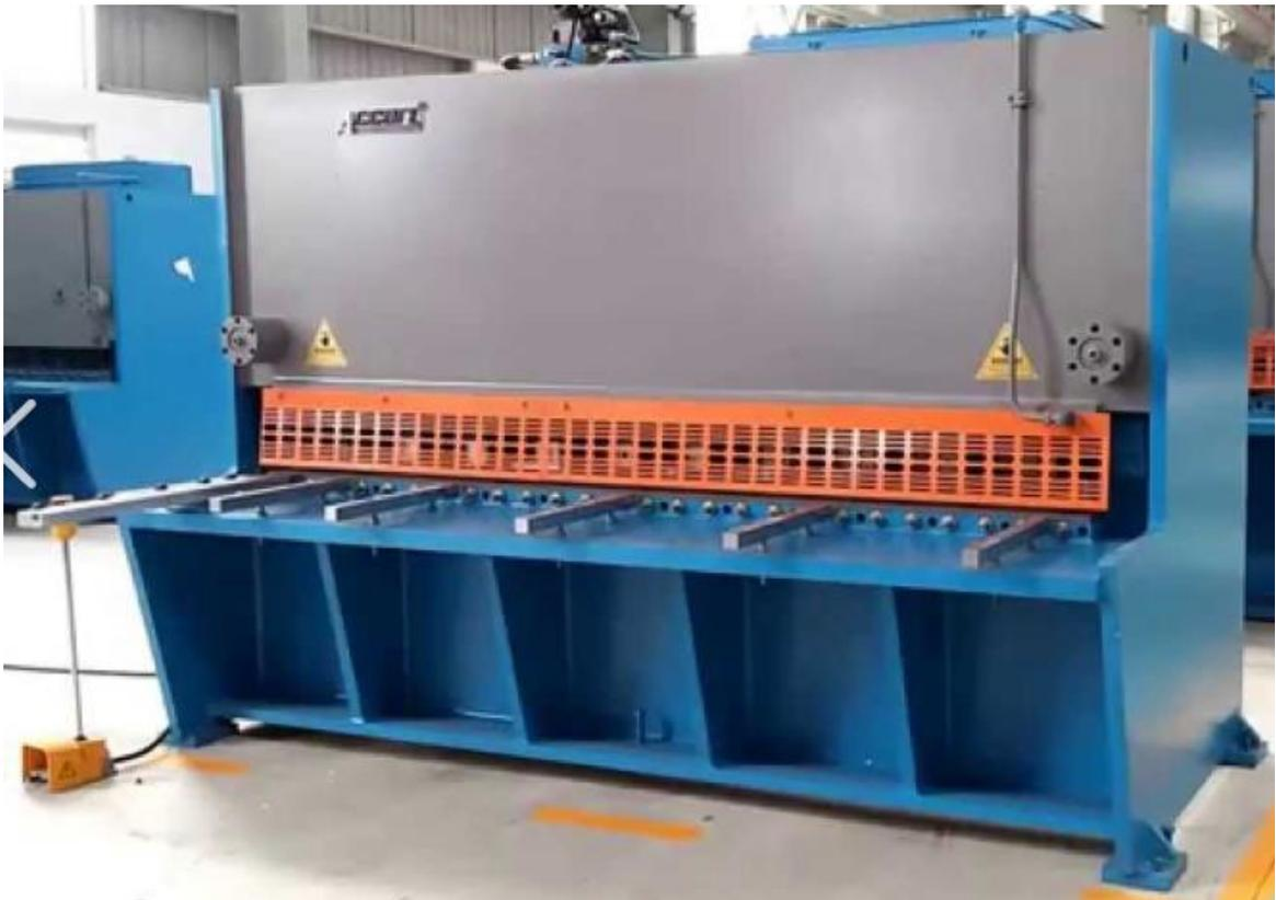
The most common guillotine injuries are crushed or amputated fingers.
